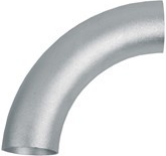
STBH Bend Elforsinket. Uten forlengede stusser. ø63–152 mm. 90°. T=2,9–4,5 mm. R= 157–380 mm.
