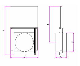
Important: the dimension of pipe line's section of feeling air has to be the same or superior to the electric valves dimensions and pressure work minimum 6 bar.
